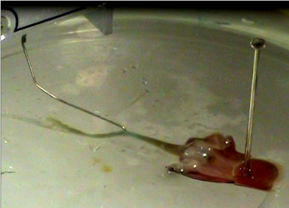
Figure 5: Isolated hindgut of the crayfish in saline attached to the hook of the force transducer
